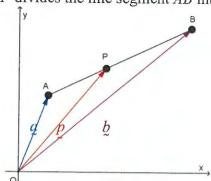
Point P divides the line segment AB internally the ratio of m:n.
